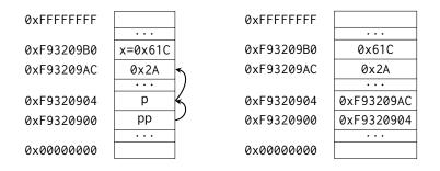
Let's assume that  $int \star p$  is located at 0xF9320904 and  $int \ x$  is located at 0xF93209B0. As we can observe:
