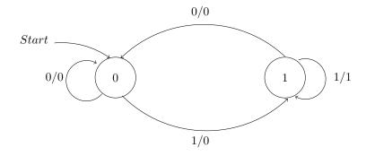
The FSM outputs a 1 if it detects the pattern "11". The FSM would output "001000000110"
