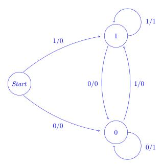
$\boxed{3.3}$  Write an FSM that will output a 1 if it recognizes the regex pattern  $\{10+1\}$ .
