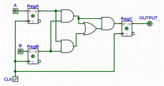
The maximum allowable hold time for RegC is how long it takes for RegC's input to change, so (clk-to-q of A or B) + CL = 4 + (5 + 5) = 14 ns.
